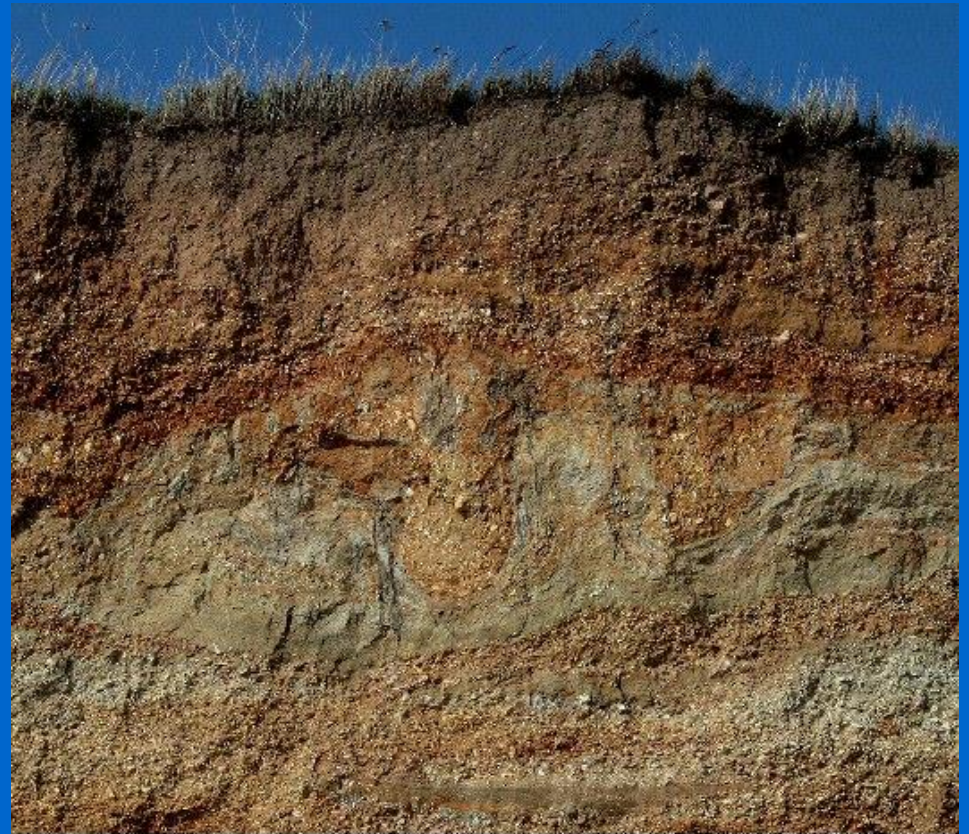
Cryoturbation in Pleistocene gravels at Chilling Cliff, Hampshire. A local lens of argillaceous sand occurs within the gravel. Pods of gravel seem to have been pushed down into the sand bed and they have a crude concentric structure. There seems to have been compaction of the argillaceous sand around the pods. Photo: 30th March 2009. Soil Work & Temp. Work (c) 2009.
